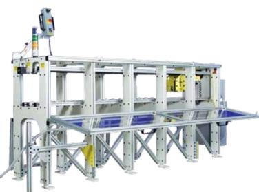
ESH-1000-S Heavy-duty fixed height shaft extractor for shafts with weights to 1100 lbs (500 kg) and lengths to 160" (4000 mm). Use in conjunction with lift table to adjust height.
