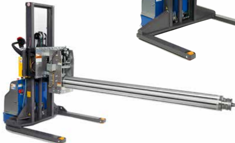
Delta HSC heavy-duty shaft handler with hydraulic lift, electric drive and hydraulic clamp. Single-stage mast with 63 (1600 mm) lift OR two-stage mast with 98 (2500 mm) lift height.
